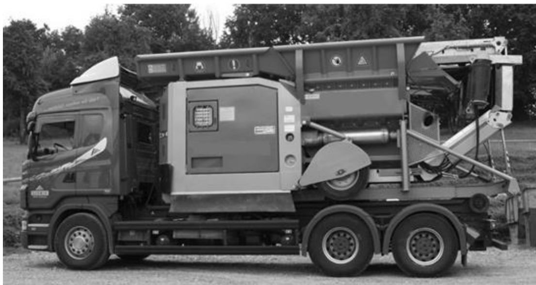
Figure 2. Two-shaft hydraulic shredder mounted on the chassis, subject of the study
