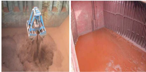
Figure 1. Iron ore fines before and after liquefaction (Tugan and Colak, 2015).
