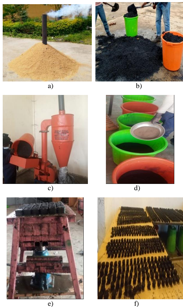
Figure 2. Process of carbonized Rice Husk Briquetting: Preparation of carbonizing of rice husk (a), cooling and storing of bio char (b), bio char grinding using a hammer mill (c), mixing of bio char powder with clay and water (d), molding of the mix using a mold maker and hydraulic jack (e), and bio char charcoal briquettes (f) (Fetene and Tikuneh, 2025)
