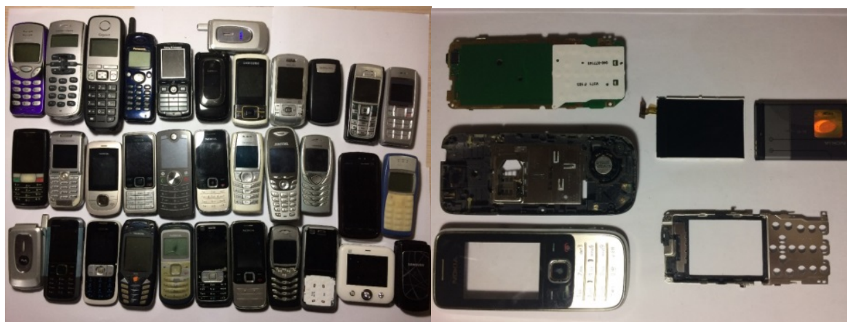
Figure 3. End-Of-Life cell phones used in the experimental study and pieces of old mobile phone after dismantling
