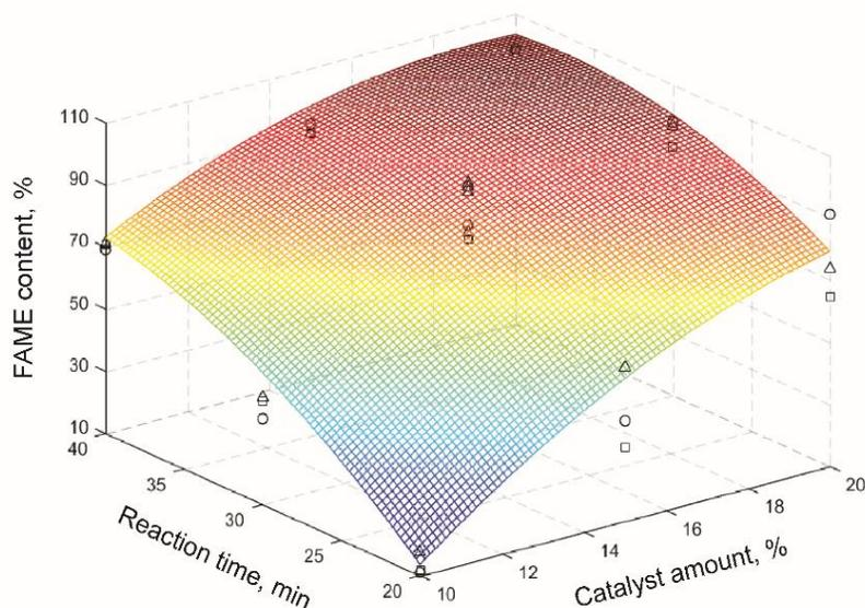
**Figure 1.** Response surface plot for FAME content as a function of catalyst loading and reaction time (surface corresponds to methanol-to-oil molar ratio of 12:1; actual FAME content at various methanol-to-oil molar ratios: 9:1 –  $\circ$ , 12:1 –  $\Delta$  and 15:1 –  $\square$ )
