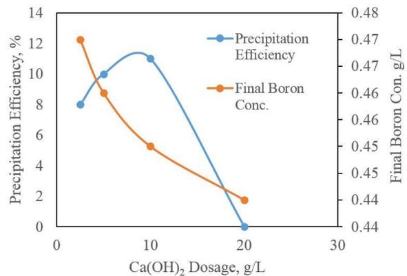
**Figure 4.** The effect of Ca(OH)<sub>2</sub> dosage on boron precipitation in the second stage
