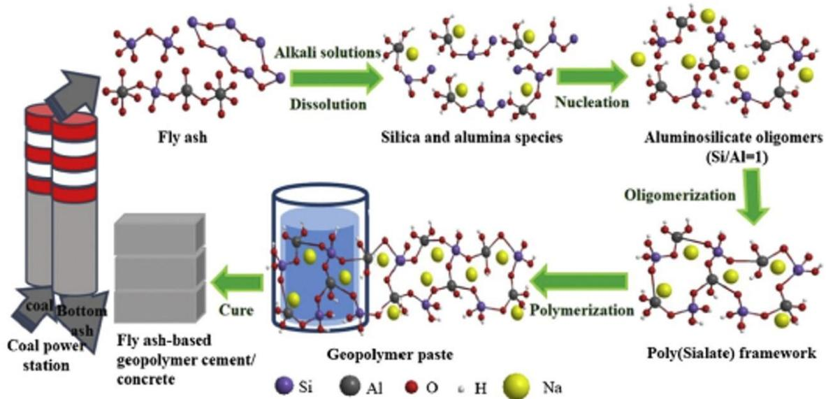
Figure 1. Geopolymer synthesis (Zhuang, 2016)
