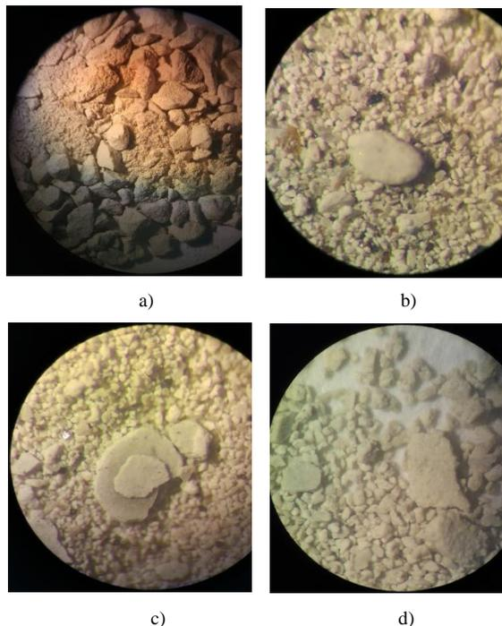
**Figure 3.** Microscopic image of zeolite samples before and after micronizing grinding: a) the initial sample obtained with the x10 magnification; b) the micronizing grinding zeolite sample after 45 seconds obtained at x100 magnification; c) the micronizing grinding zeolite sample after 120 seconds obtained at x100 magnification; d) the micronizing grinding zeolite sample after 900 seconds, obtained at x100 magnification
