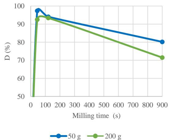
**Figure 2.** Cumulative mass of the bulk class (- 5 + 0)  $\mu\text{m}$  depending on the grinding time
