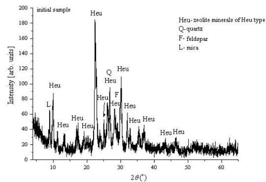
**Figure 1.** XRD analysis of the initial sample of zeolite
