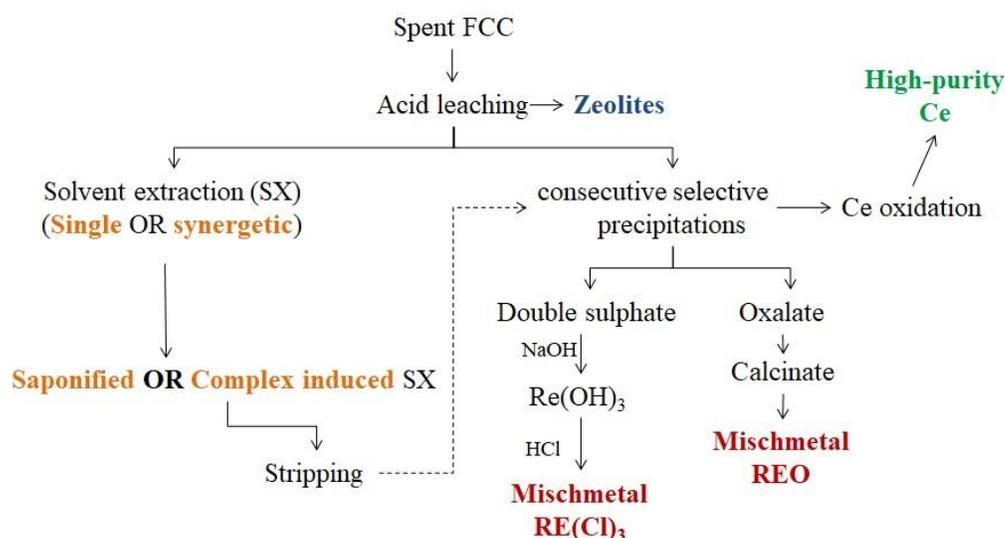
**Figure 2.** Schematic flowsheet for complete recovery of REE from spent FCC. Legend: Green – final, highly pure products for reuse; Red – final low purity products ready for reuse; Blue – potentially reusable wastes
