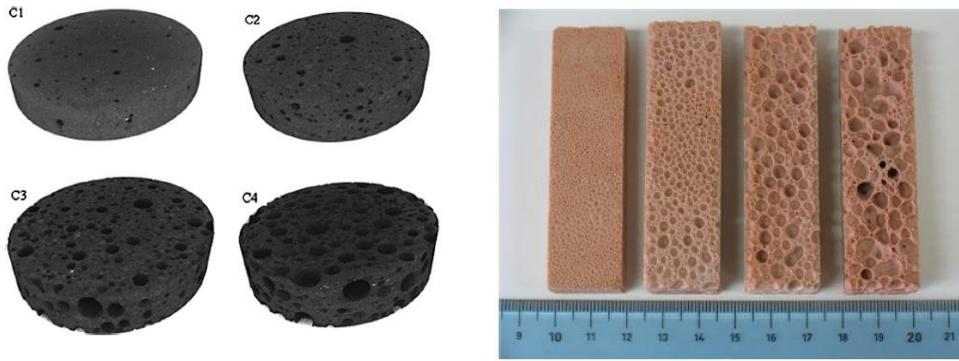
**Figure 2.** Geopolymer foams with different a) Al content c1-c4=5, 10, 15, 20 mg Al powder, 100 ml alkali solution, c4=70 % porosity (Zhang et al., 2014), b) H<sub>2</sub>O<sub>2</sub> content, 1,2,4,6 wt %, H<sub>2</sub>O/Na<sub>2</sub>O=13 (Palmero et al., 2015)
