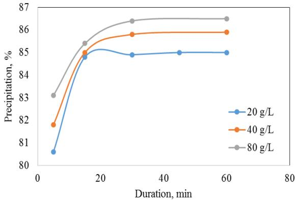
**Figure 2.** The effect of agitation duration on boron precipitation with different Ca(OH)<sub>2</sub> dosages
