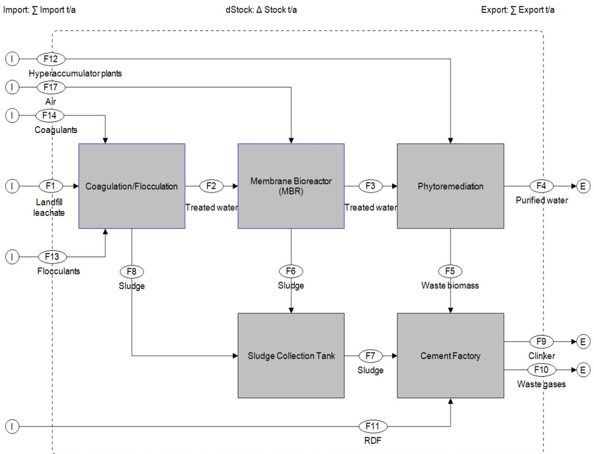
Figure 6. Model of a landfill leachate treatment plant
