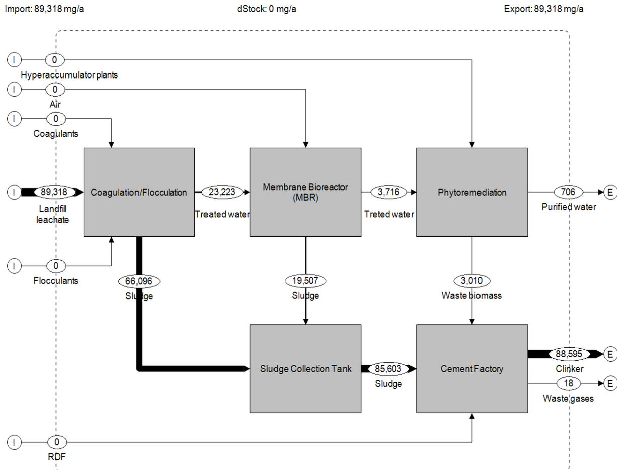
Figure 12. The flow of cadmium within the process of filtering leachate from municipal solid waste landfills in an adequate plant for physical and chemical, biological and alternative treatment (mg/year)
