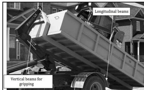
Figure 3. Chassis construction type
