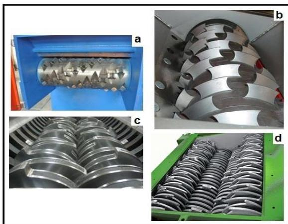
**Figure 1.** Different types shredders (Vatskicheva and Grigorova, 2017a)
