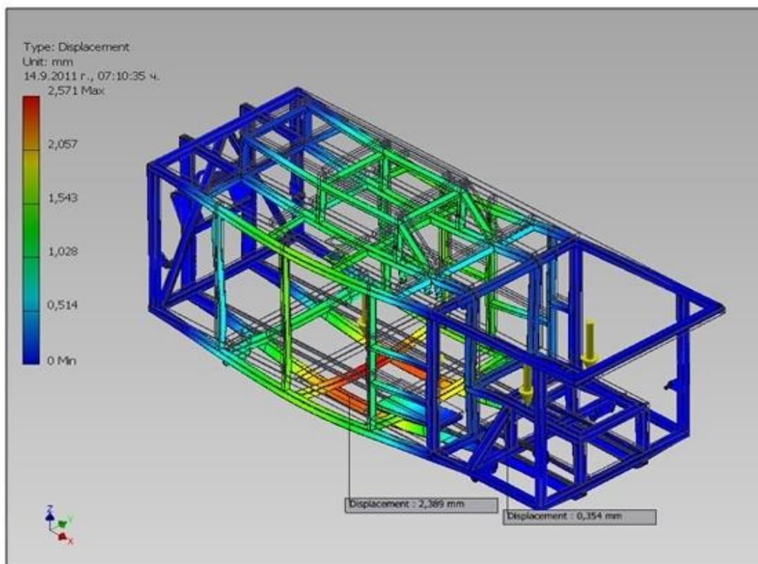
**Figure 5.** Data for frame maximum and minimum deformations
